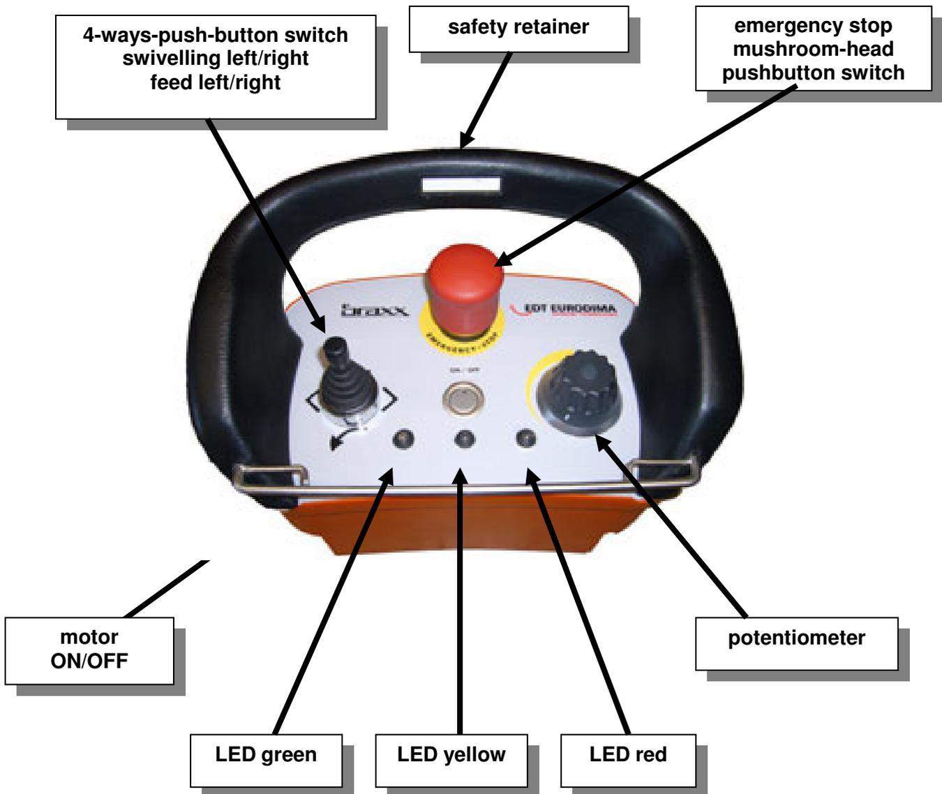
In general, this remote control is to be used for steering the wall saws tornado SB321 and typhoon SB200. For the wire saw WB12, no remote control is necessary. Therefore, the emergency stop plug (located in the tool case) must be plugged to the remote control connection.
