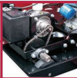
Heavy-duty hydro static transmission with variable speed drive
