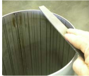
Degrease & file tube surface
