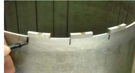
Marking tube for even spacing
