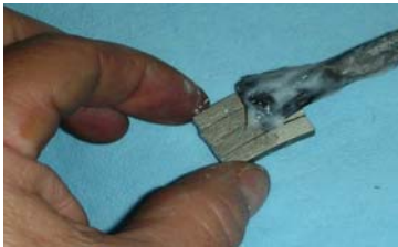
Apply flux to the un-marked side of segment.
