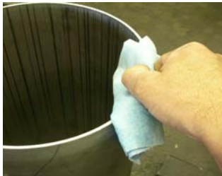
Degrease & file tube surface
