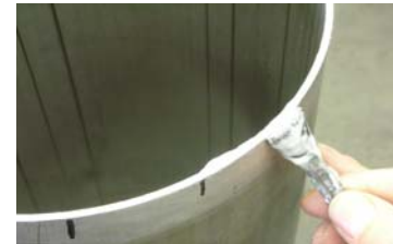
Apply flux on the tube
